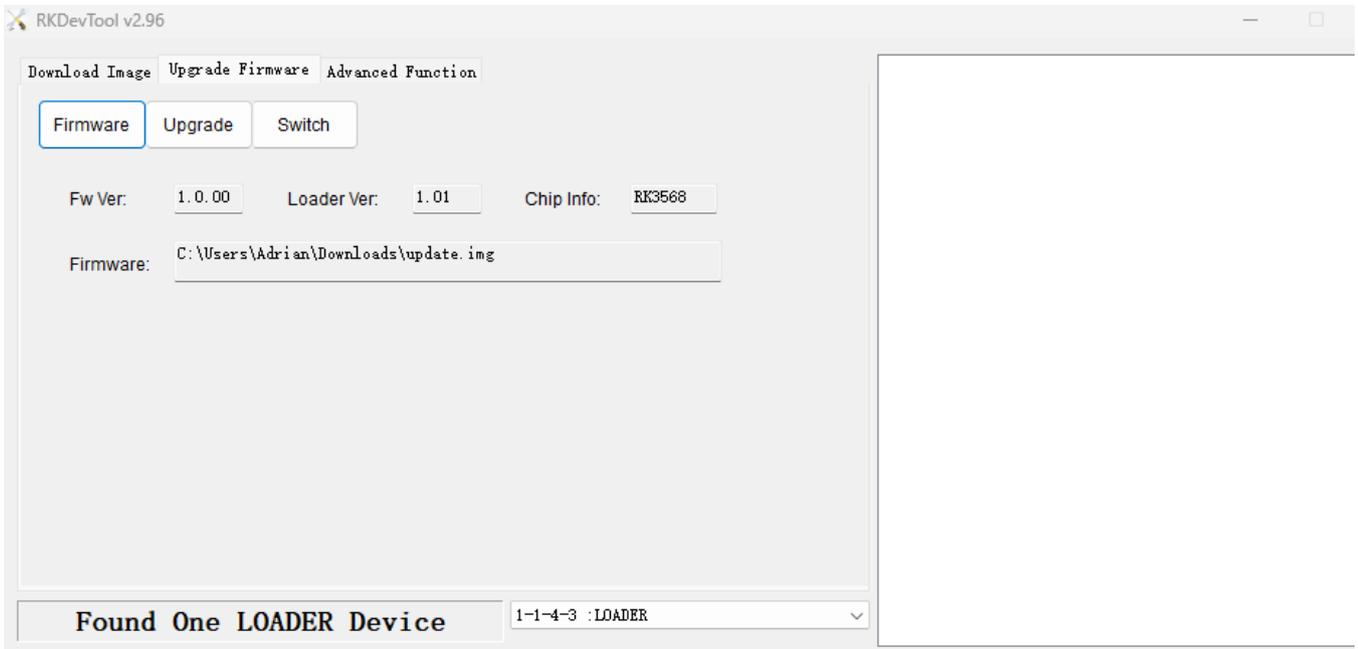
4. Click *Upgrade* to reinstall operating system. After few minutes device is ready. Upgrade should end with *Download Firmware success* message. Device should automatically reboot.
